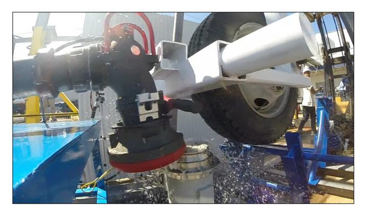
**Costa Mesa, California, September 25, 2015** – On September 25<sup>th</sup>, 2015, the qualification test for Cla-Val's hydrant coupler (353GF-3) was witnessed by a representative of the Energy Institute to validate the coupler's compliance with **El 1584, 3rd edition**. The coupler successfully passed all required tests. Cla-Val's 3<sup>rd</sup> Edition Pressure Control Couplers are now available for purchase through our global distribution partner, Parker Velcon.
